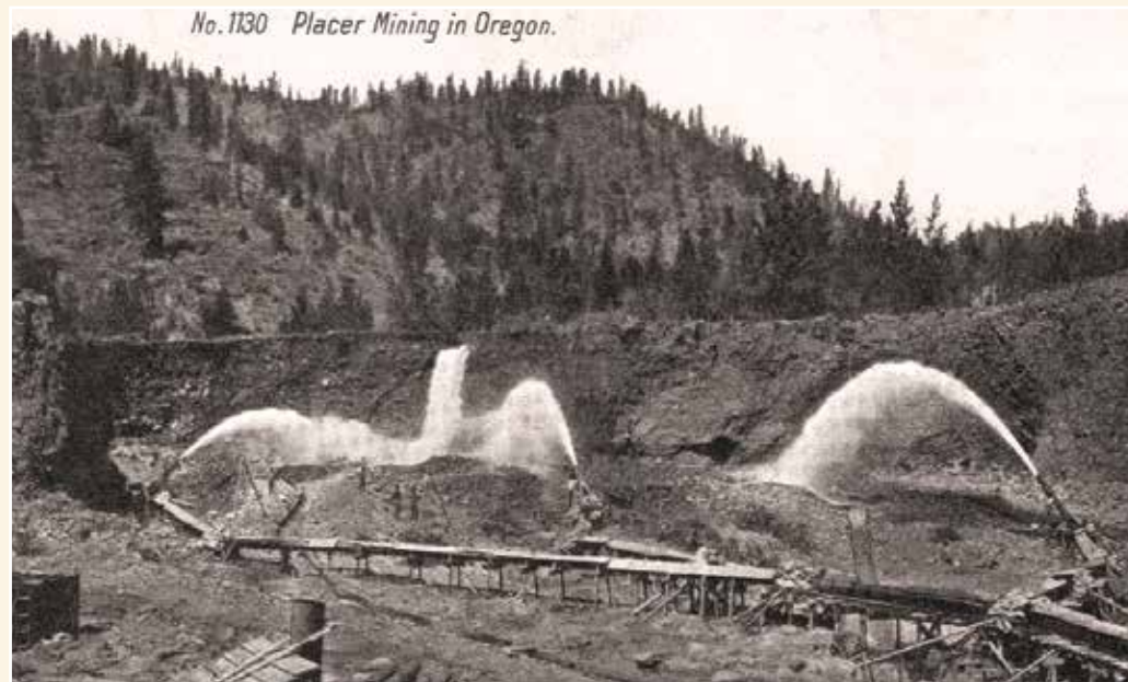
Hydraulic (Placer) mining at Sterling Creek Mine, 1905. Photo: Southern Oregon Historical Society.
